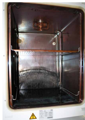
Figure 2. Appearance of a pure copper incubator after several years of activity.
